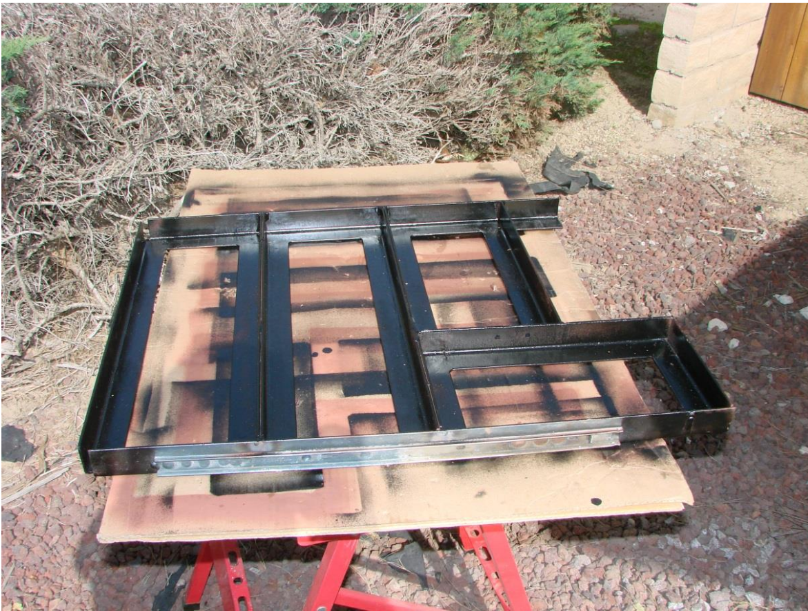
Two views of the revised tray. Note the 1.75" extension at the far right.
